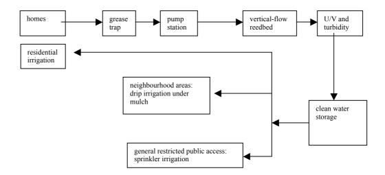
Conceptual plan of effluent system components
